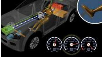
XH drive uses ultracaps to accelerate, protecting batteries from deep-cycle damage
